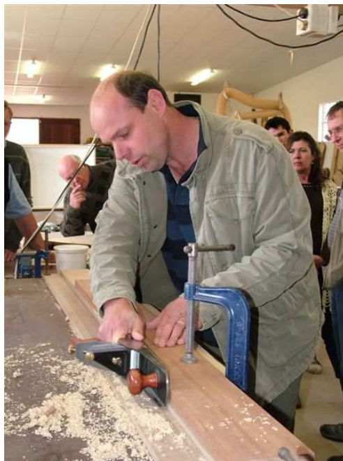
Trimming veneer edges in a shooting board The plane is a very sharp Veritas Plane
