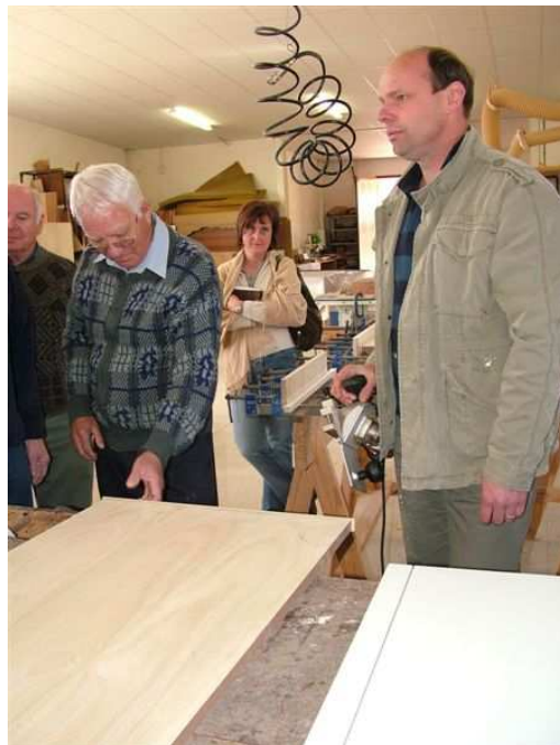
Edge trimming the veneered door
