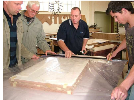
Vacuum press Note taped sides of sheets
