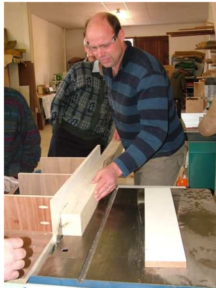
Sawing jacaranda veneer with a rip blade Note use of safety glasses
