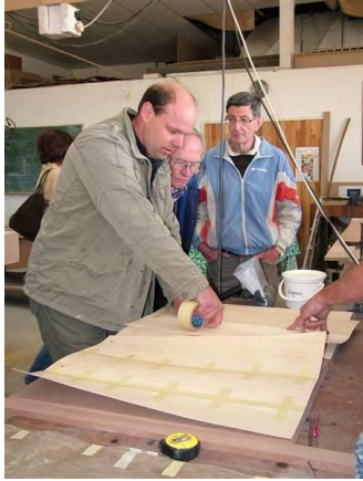
Taping selected veneer sheets together
