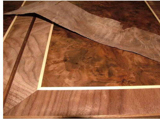
Detail of walnut veneering and inlay work
